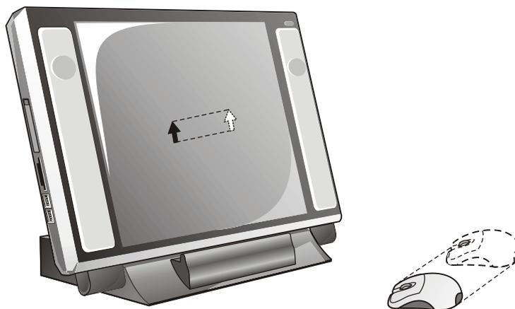
To use the mouse, slide it on a clean, flat surface (such as your desktop) and the pointer on the screen moves accordingly.
