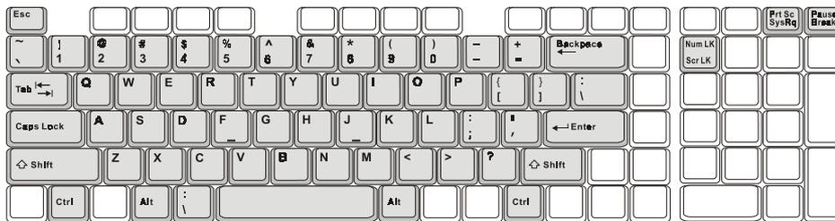
Typewriter keys are similar to the keys on a typewriter. Several keys are added, such as the **Ctrl**, **Alt**, **Esc** and lock keys, for special purposes. When the lock keys are pressed, their corresponding indicators light up.
